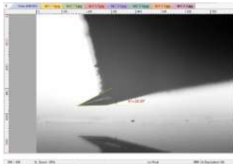
Figure 2. Accessory chart, for reference only. Angles are based on stiff, 200um sapphire bare fibers. For softer materials, angle may change due to the ferrule protrusion limits of fiber's material.
