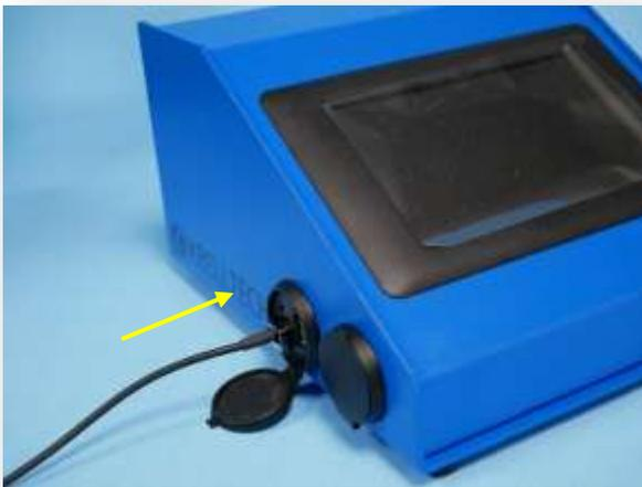
2. Insert coning module into designated Orbit port, as shown.
