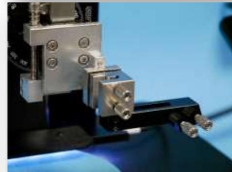
5. Place entire coning module into adapter. Set angle and check protrusion lengths using profile scope.
