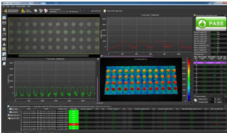
MPO-48 PC endface measurement example.
