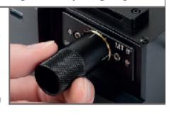
Adjusting Ring clockwise to cut closer to the ferrule face, counterclockwise to cut further away. Each calibration mark on the Adjusting Ring represents a 25 µm distance. The cut distance can be set between calibration marks for an even finer adjustment.
