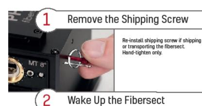
Press and hold Start Button to turn on the fibersect. Release when the READY light turns red. The READY light will then turn green, indicating that it's ready for use. The fibersect will turn
