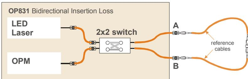
Switch the instrument to Ref mode and press the Ref button to execute the referencing cycle. The instrument will cycle through all the wavelengths in A-B and B-A direction, takes the absolute power reading and stores them. The instrument will end up in A-B mode at the end of this process.
