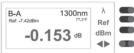
Other cables can be measured by simply connecting them to the two reference cables as shown above. There is no need for a repeated reference cycle unless the reference cables have been changed. If a long time (hours) has elapsed since the last reference cycle or the measurement procedure requires a frequent referencing.
