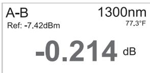
To measure the insertion loss in the other direction use the mode button to switch to B-A mode. The display of the B-A measurement will show the insertion loss of the connected cable. To measure and display the insertion loss at the other wavelength (if available) use the wavelength button and switch the wavelength.
