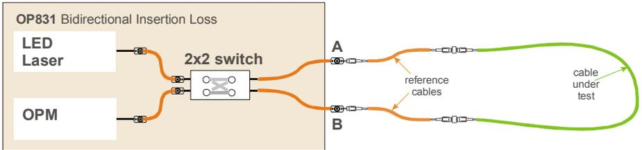
The display of the A-B measurement will show the insertion loss of the connected cable. To measure and display the insertion loss at the other wavelength (if available) use the lambda button and switch the wavelength.
