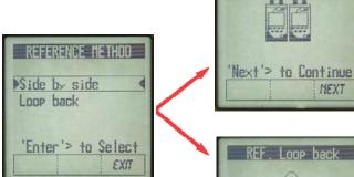
Side by side reference is selected when both units are together and referencing can be accomplished. This method is more accurate due to cross calibration of units.
