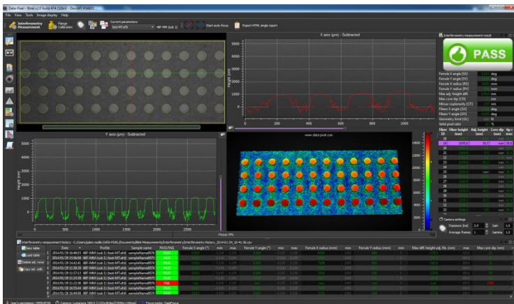
MPO-48 PC endface measurement example.
