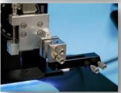
5. Place entire coning module into adapter. Set angle and check protrusion lengths using profile scope.
