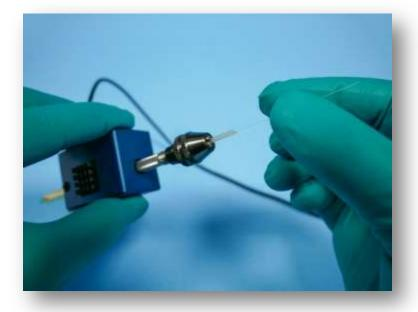
4. See figure 2 to choose correct Angle extender. Loosen thumbscrews and insert designated extender. Place flat towards thumbscrews. 3. Loosen collet and insert bare fiber. Set estimated protrusion length and tighten collet. Fiber protrusion lengths may be better set while on the machine with aid of the profile microscope. Tip: Spin the fiber as it's guided through the ferrule. This is especially true when loading the extended Fiber Adapter
