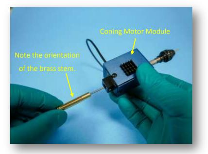
3. See figure 2 for choosing correct adapters and insert into the coning motor module. Tighten locking screw with 0.05" driver. Note: Do not remove the steel fiber guides, as they are set to designated heights.
