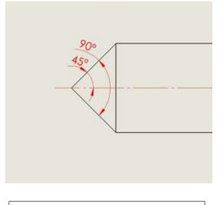
Figure 1a. Use as reference to figure 2. To Polish a **90° Cone**, set polishing angle to 45 °
