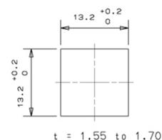
Figure 4 Cut-hole dimensions
