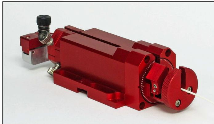
For determining angular movements, the rotator is equipped with a graduated dial marked at 10-degree intervals.
