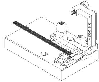
Shown is the fiber array holder with a 16 fiber array
