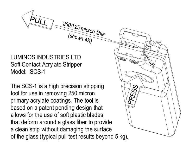
DIRECTIONS: Place the coated fiber between the contacting edges of the plastic blades. Press <u>firmly</u> with your thumb on the Logo (shown in "right-handed" orientation above). Pull the fiber in the direction shown and the coating will peel away from the fiber as depicted above. The plastic blades are a low-cost user replaceable part with an average lifetime of many thousands of strips per pair.
