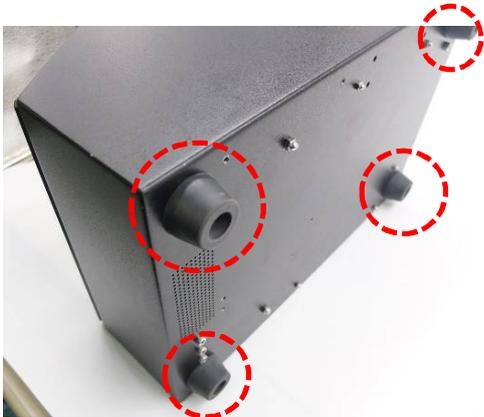
2) Tilt down the Polishing machine and remove the rubber feet. The rubber feet are secured with hexagon socket head cap screws. Tilt the Polishing machine to the side.
