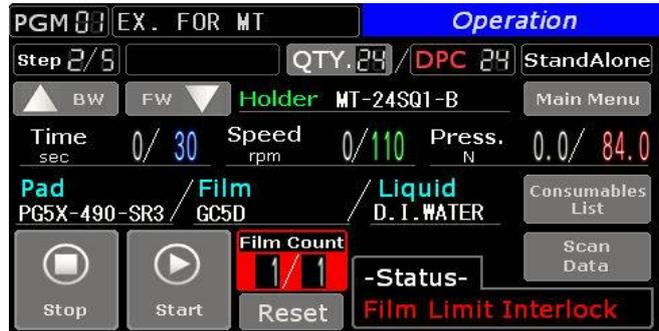
you can not proceed polishing unless reset the film usage. Long press of Rest will allow to reset film usage count of this step. In case you want to disable the film usage counting, please enter the life as 0. Also you can disable the film usage Interlock on the Configuration.
