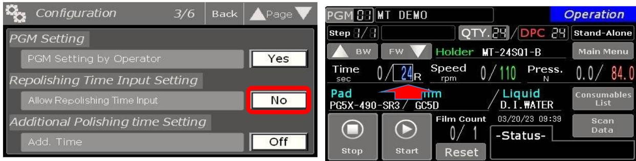
When the setting is set to "Yes," a white frame will be added to the time display on the operation screen to allow selection. Once selected, numeric keypad will be displayed, allowing you to enter the polishing time and fine-tune the polishing amount as necessary.
