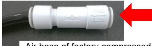
Air hose of factory compressed air is connected to this end; make sure to supply dry air meets the specification
