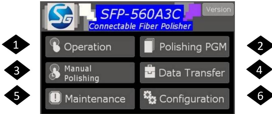
The main menu consists of six functions: "Operation," "Polishing PGM," "Manual Polishing," "Data Transfer," "Maintenance" and "Configuration." The following sections explain how to operate each function.
