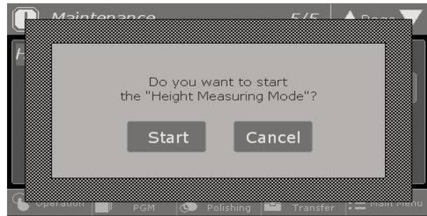
After the measurement is done, press Stop and then the turntable will go back to the original position.
