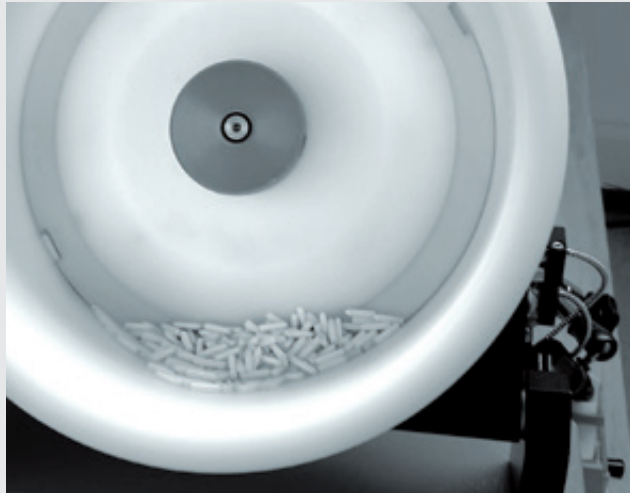
The workpieces are filled into a drum feeder and led to the handling station
