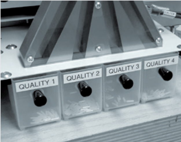
After measuring the work pieces are sorted into 4 quality classes
