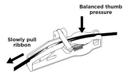
Apply gentle thumb pressure to add drag. Pull ribbon along arc towards blade edge to slice matrix. Slice 1 matrix node every 5 seconds or slower.
