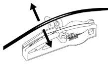
Carefully separate ribbons at load location. Load around and under blade edge. Do not break matrix.
