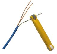
2. Continue turning the guide roller and allow the tool to self feed and unwind the twisted pair.
