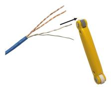
3. Press the guide roller and slide the tool off the unwound twisted pair to straighten them.
