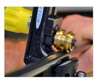
Accommodates a wider range of cable diameters without additional guide wheels.
