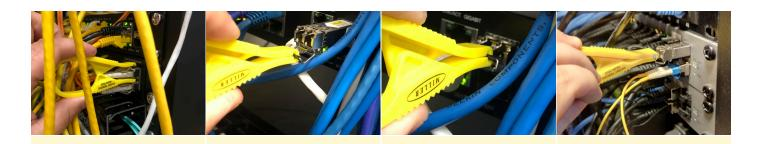
Engage the tool with the transceiver latch
