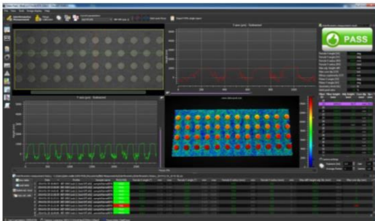
MPO-48 PC endface measurement example.
