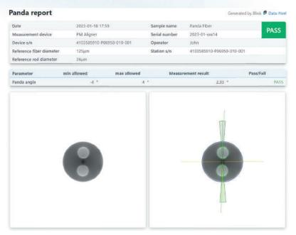
Blink software detects automatically the stress rods regardless of their shapes (circular, hexagonal,...) and allows a precise alignment of PM fibers.
