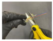
6. The KS-2 shears are good for any Kevlar strength fibers.
