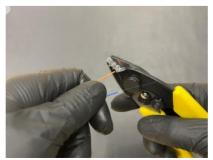
5. Use the smallest notch on the CFS-3 for individual fiber, or largest notch for flexible buffer tube.
