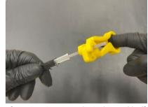
3. After trimming away the jacket and buffer tubes, ring twice with the FTS scoring tool.
