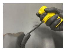
2. Use the MB04 Twister drop slitter to score each side and peel away the jacket.
