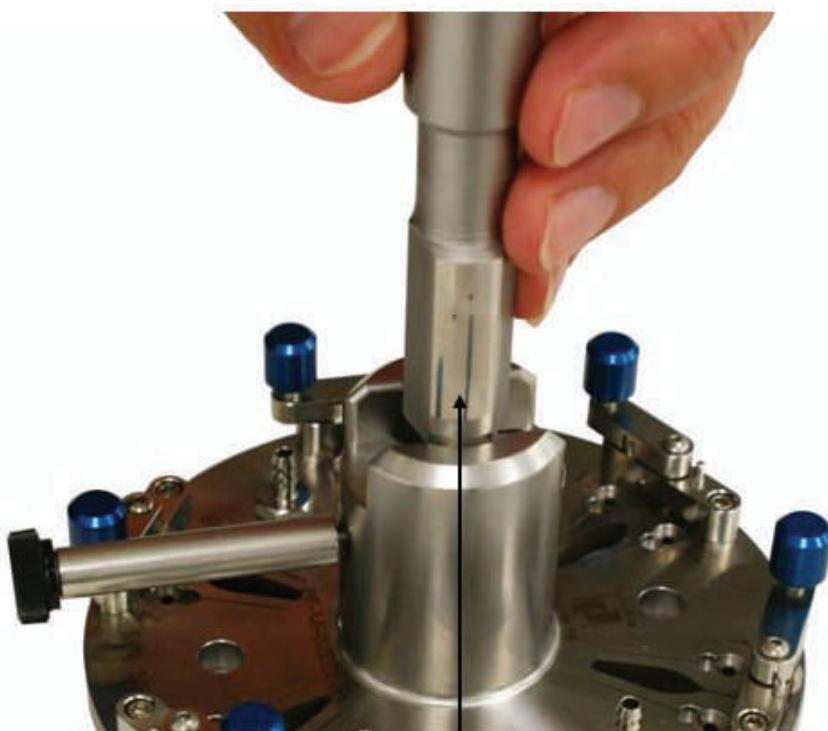
Gently engage diamond end of Fixture Bore No-Go Gage into center fixture hole. If gage goes in, fixture needs replacement
