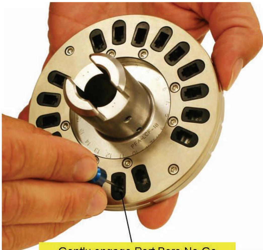
Gently engage Port Bore No-Go Gage into port fixture hole. If gage goes in, fixture needs repair or replacement. All ports in fixture need to be checked.
