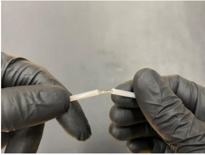
3. Snap the buffer tube to expose the inner fibers. Clean if necessary.
