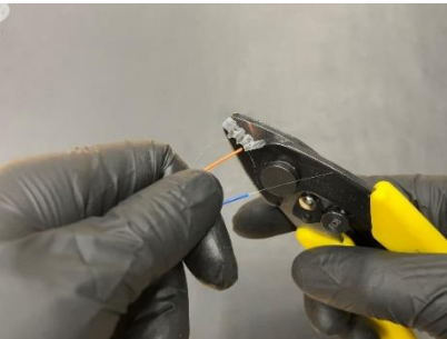
4. Use the smallest notch on the CFS-3 for individual fiber, or largest notch for flexible buffer tube.
