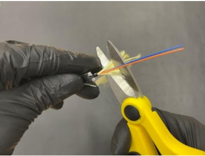
5. The KS-2 shears are good for any Kevlar strength fibers.
