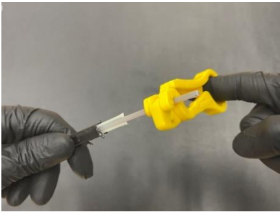
2. After trimming away the jacket, ring twice with the FTS scoring tool.
