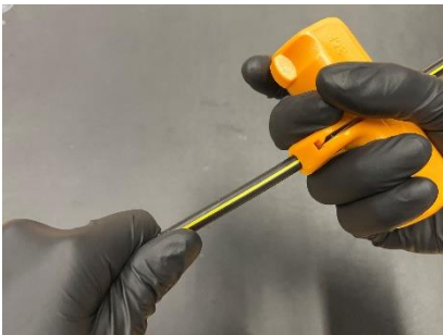
1. Use the MB04 ULW Twister drop splitter to score each side and peel away the jacket.
