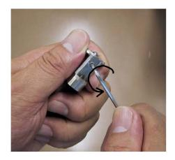
Step 2 Remove the jig mounting block bolt with an Allen wrench.
