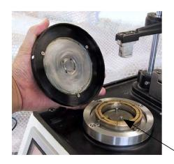
Step 6 Fit the base disk to the guide pins.
