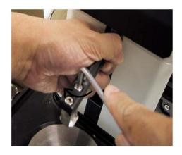
Step 6 Install the jig mounting block bolt with an Allen wrench in the reverse order of Step 1.
