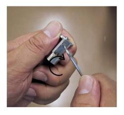
Step 5 After adjustment, insert the set screw into the jig mounting block and install the jig mounting block with an Allen wrench in the reverse order of Step 2.
