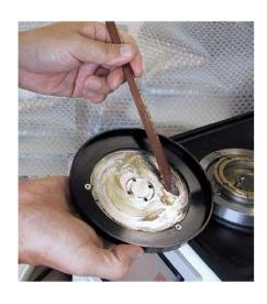
Step 5 Also coat the rear side of the base disk with the accessory grease using a bamboo spatula, etc.
