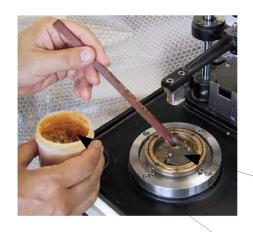
Step 4 Coat the drive shaft and its surrounding area with the accessory grease using a bamboo spatula, etc.
