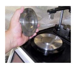
Step 7 Install the polishing disk.
