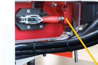
To adjust the drive belt tension: turn the adjustment screw (hex screw M6) counterclockwise to tighten the drive belts or clockwise to reduce tension. The expansion arm increases tension when placed in position. Check the tension of the drive belts until the correct tension is achieved.
