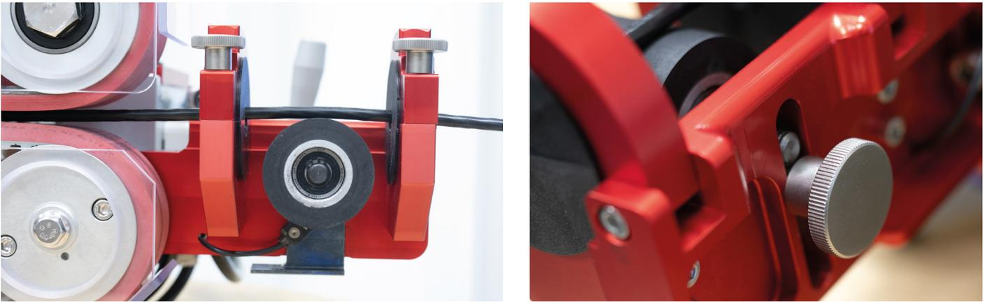
2. Thread the cable through the rear cable guide and between the belt drives to check mobility.
