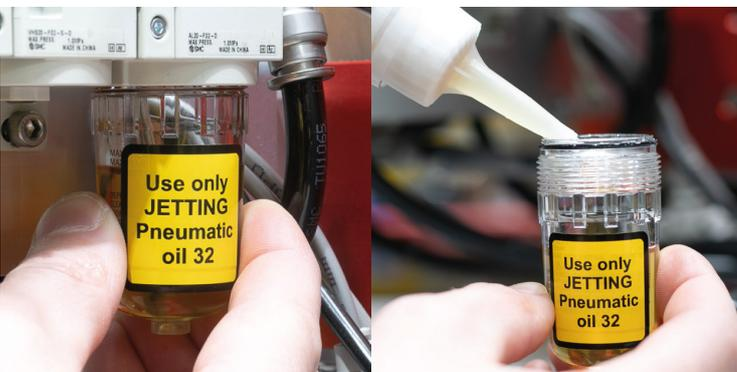
**Alternative 2.** Unscrew the entire container by hand counterclockwise and pour the oil directly into the container.
