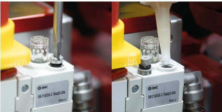
**Alternative 1.** Loosen the oil container screw and fill.
