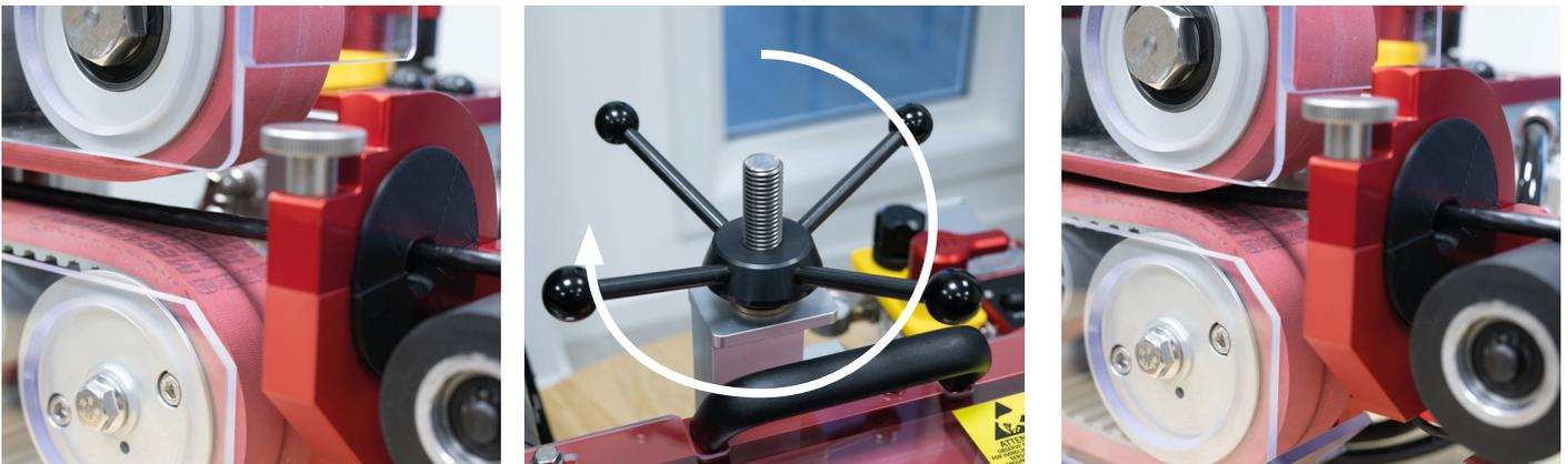
3. Tighten the upper and lower drive units with the Belt Clamping Lever to ensure even pressure on the cable.
