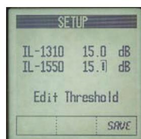
User has the ability to select 1310, 1550nm or 1310 and 1550nm testing.
