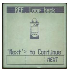
Loop back referencing method is chosen when the units are separated and it is not convenient to co-locate instruments.
