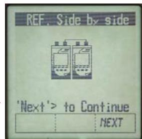
Side by side reference is selected when both units are together and referencing can be accomplished. This method is more accurate due to cross calibration of units.
