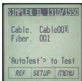
Instrument automatically assigns file name. User may select base name in start # and increment amount.
